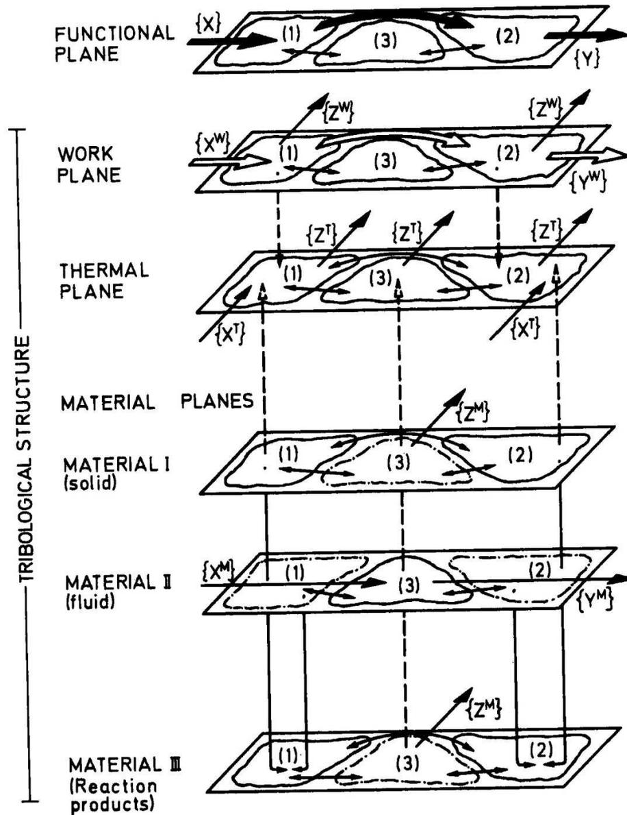
Figure6: The Tribo-process diagram: Conceptual planes of parameters and Processes in a tribo- mechanical system.
