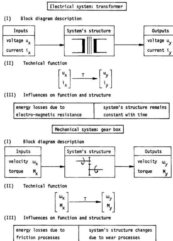
Figure 3: Comparison of the characteristics of an electrical and a mechanical system.
