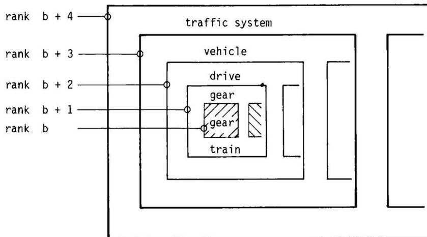
Figure 1: Example of a hierarchy of systems.
