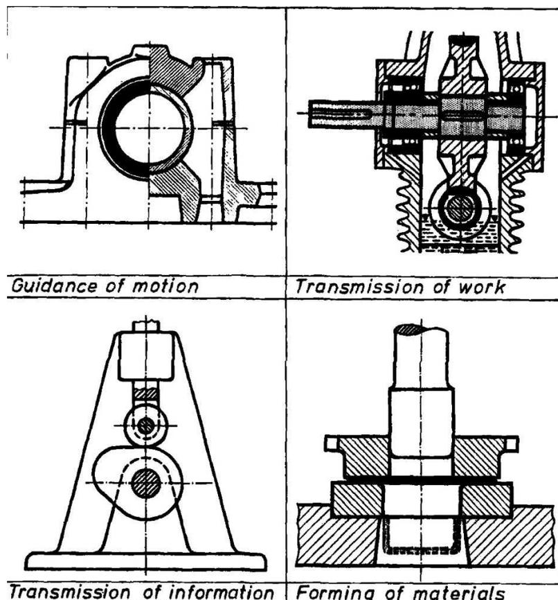
Figure 4: Types of tribo-mechanical systems
