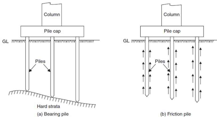
Fig. 11 Pile foundation a) End bearing piles; b) Friction piles
