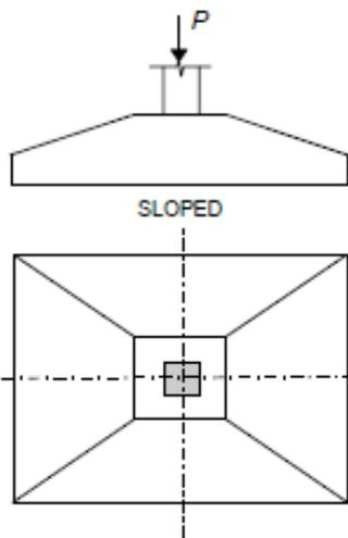
Fig. 3 Sloped footing
