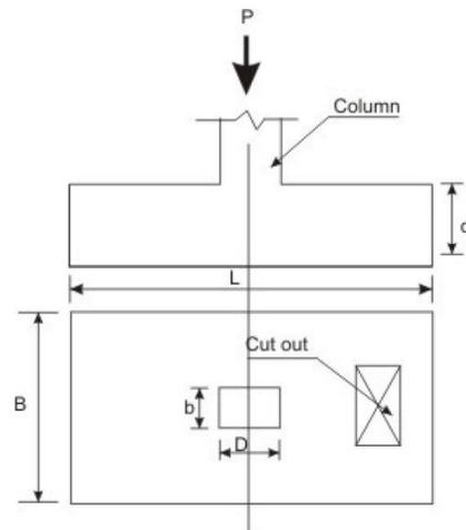
Fig. 4 Unsymmetrical footing about x-axis
