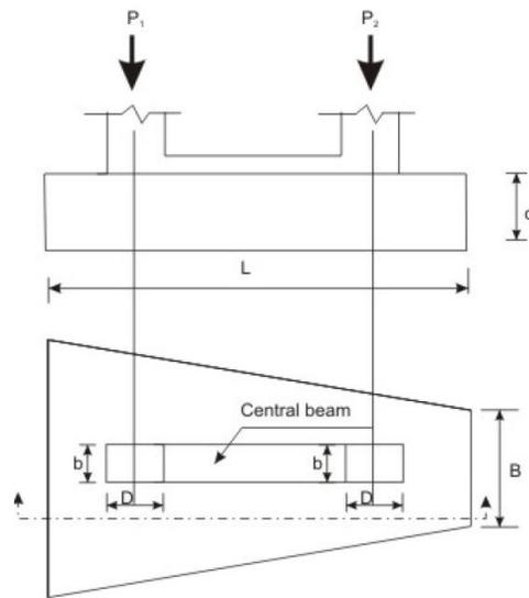
Fig. 5 Combined footing without a central beam    Fig. 6. Combined footing with a central beam
