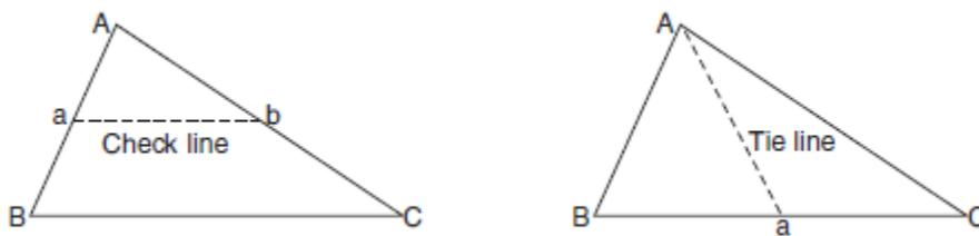
**Fig. 1.4 Check line and tie line**
