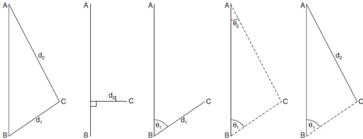
**Fig. 1.3 Locating point C w.r.t. points A and B**
